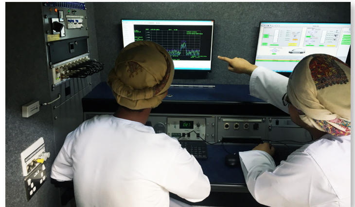
TRA of Oman's staff in the RF monitoring vehicle locating the source of interference.
