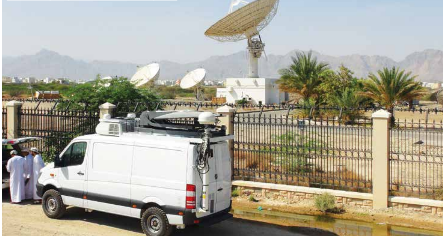
The TRA on a regulatory mission with the RF monitoring vehicle.
