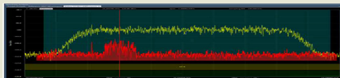
▲ Carrier-under-Carrier display within satID to identify interference.
